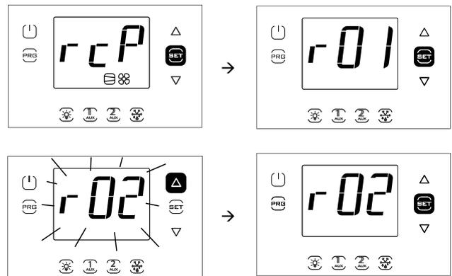
**Note:** the figure refers to the screens on models with single row display, P/Ns WB000S\*. In models with two rows, P/Ns WB000D\*, as well as the message indicated, during navigation the display shows the scrolling message "bni - recipe index now active" on the second row.
