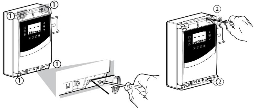
3.b: Fasten the screws (1) and fix the panel. Loosen the screws (2) and open the panel.
