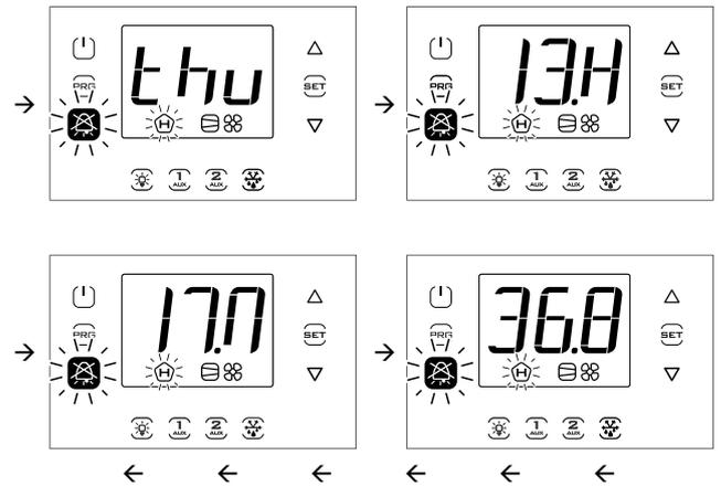
**Note:** the figure refers to the screens on models with single row display, P/Ns WB0005\*. In models with two rows, P/Ns WB000D\*, as well as the message indicated, during navigation the display shows the scrolling message "HACCP Alarms" on the second row.
