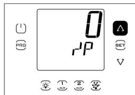
5. Press Set: the second row of the display will scroll the code and description of the first parameter in the category: /21 – Probe1 meas. stab.; the first row of the display will show the current value of the parameter
