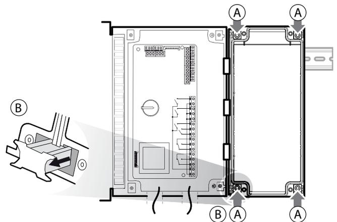
4: Put the module close to UltraCella control and insert the coupling clamps supplied as standard.
