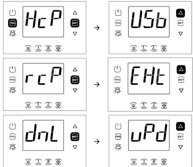
**Note:** the figure refers to the screens on models with single row display, P/Ns WB000S\*. In models with two rows, P/Ns WB000D\*, as well as the message indicated, during navigation the display shows the scrolling message "recipes in USB device" on the second row.
