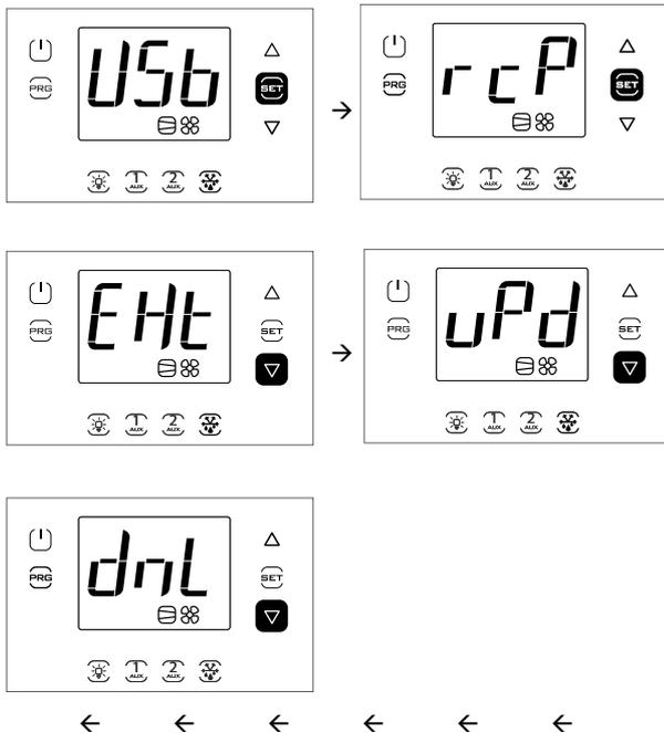
Note: the figures refer to the screens on models with single row display, P/Ns WB000S\*. In models with two rows, P/Ns WB000D\*, as well as the message indicated, during navigation the display shows the scrolling message "recipes in USB device" on the second row
