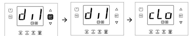
**Note:** the figure refers to the screens on models with single row display, P/Ns WB000S\*. In models with two rows, P/Ns WB000D\*, as well as the message indicated, during navigation the display shows the scrolling message "Digital input 1 status" on the second row.
