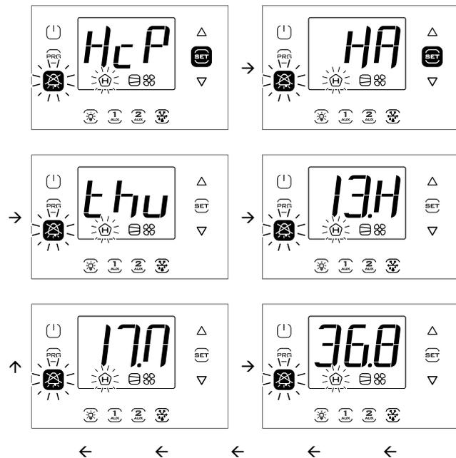
**Note:** the figure refers to the screens on models with single row display, P/Ns WB000S\*. In models with two rows, P/Ns WB000D\*, as well as the message indicated, during navigation the display shows the scrolling message "HACCP Alarms" on the second row.
