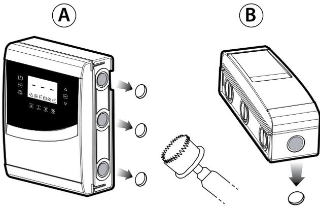
1: Use a hole saw to drill the panel in correspondence with the predrilled holes (steps A, B). If present, fasten the DIN rail for the module.
