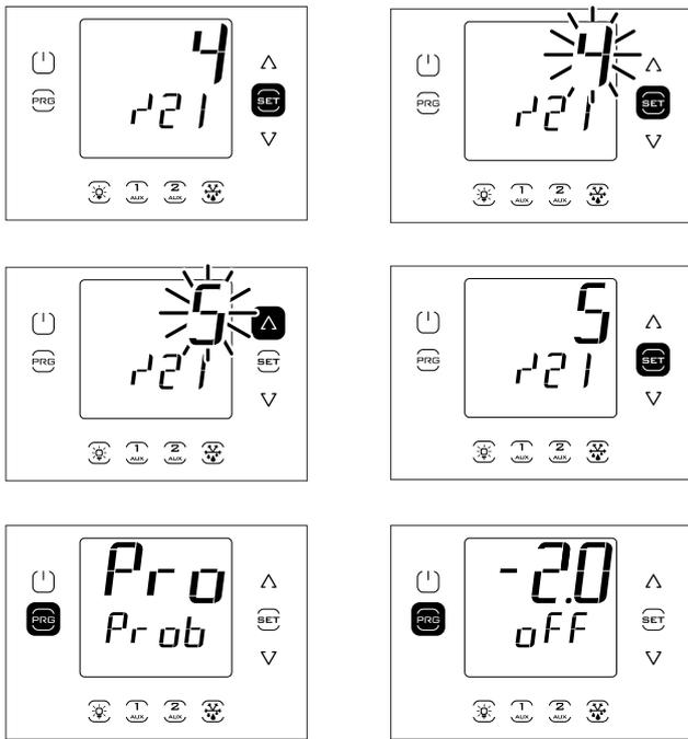
**Note:** in the parameters or set point modification procedures, the new value is saved every time the Set key is pressed.
