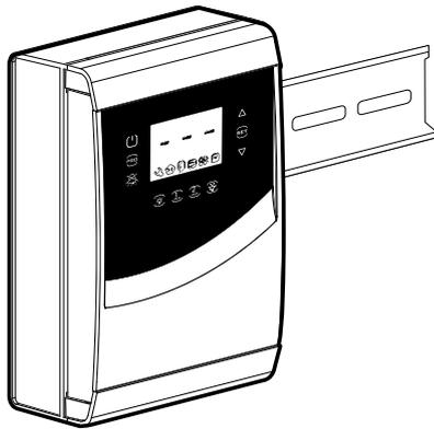
1.a: Fix the DIN rail and insert the controller
