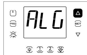
6. press SET to confirm the download of the saved alarms. The message "ALG" will flash during the download procedure; at the end, "ALG" will stop flashing and the green LED next to the USB port will come on, indicating the end of the procedure; if for some reason the procedure
