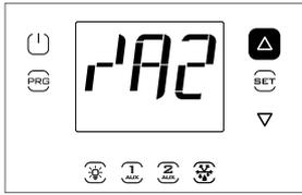
10. Press UP to move to parameters /A2.../ A5; make any required settings.
