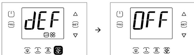
**Note:** The Figures refer to the screens on models with single row display, P/Ns WB000S\*. In models with two rows, P/Ns WB000D\*, the message "Off" appears on the second row of the display.
