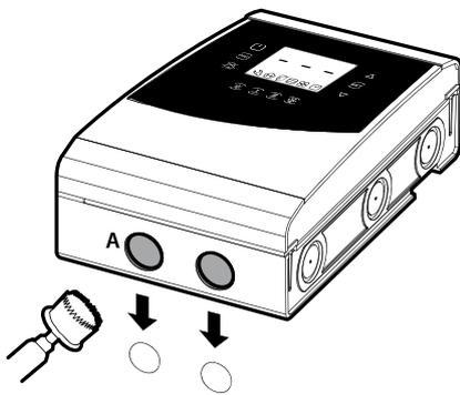
4: Use the holes and mount the cable glands to connect:
