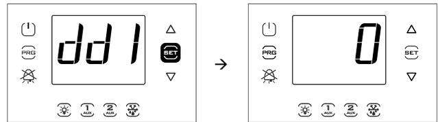
**Note:** the figure refers to the screens on models with single row display, P/Ns WB000S\*. In models with two rows, P/Ns WB000D\*, as well as the message indicated, during navigation the display shows with a scrolling message, parameter code and description: "dd1 - defrost1-day"
