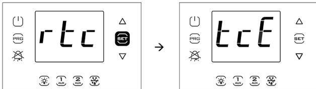
**Note:** the figure refers to the screens on models with single row display, P/Ns WB000S\*. In models with two rows, P/Ns WB000D\*, as well as the message indicated, during navigation the display shows with a scrolling message, parametercode and description: "tce - enable data modification".
