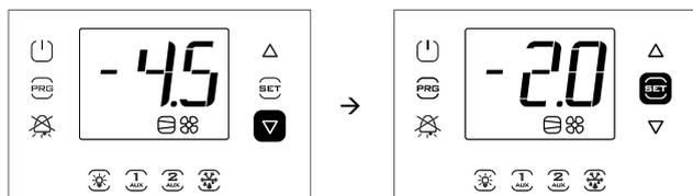
**Note:** the figure refers to the screens on models with single row display, P/Ns WB000S\*. In models with two rows, P/Ns WB000D\*, as well as the message indicated, during navigation the display shows the scrolling message "Setpoint" on the second row
