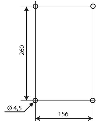
1.b: Make 4 holes (Ø 4,5 mm) according to the drilling template and insert the dowels (mm)
