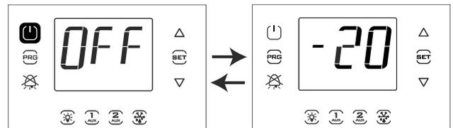
1. When first starting, the controller is OFF.
