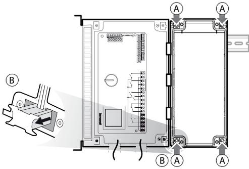
3.a: Mark on the wall the positions of the lower holes, remove the panel and perform the drills (Ø 4.5 mm); insert the plugs. Replace the panel on the DIN guide and fix it fastening the lower screws.
