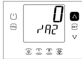
9. Press UP to move to par. /A2.../ A5; make any required settings.
