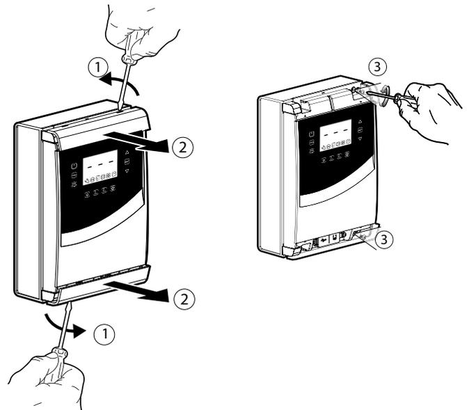
2: Remove the faceplates. Unscrew the screws (3) and open the UltraCella control
