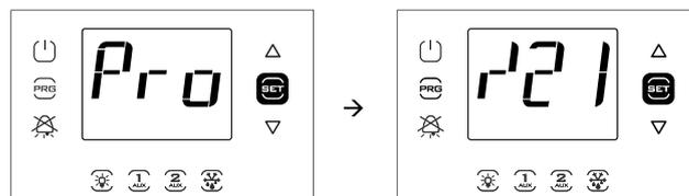
**Note:** when setting the parameters or the set point, the new value is stored whenever the Set button is pressed.
