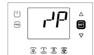
9. Press Set to confirm and return to the parameter code. The new value has now been saved on the controller.
