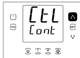
11. Press UP to move to category CtL (the second row scrolls the name of the second category of parameters: Control) and follow the previous steps to set St and the subsequent parameters, as shown in the previous table and in the parameter table.
