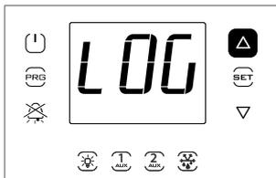
**Note:** the figure refers to the screens on models with single row display, P/Ns WB000S\*. In models with two rows, P/Ns WB000D\*, as well as the message indicated, during navigation the display shows the scrolling message "recorder" on the second row.
