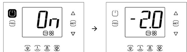
**Note:** The Figures refer to the screens on models with single row display, P/Ns WB000S\*. In models with two rows, P/Ns WB000D\*, the message "On" and "Off" appear on the second row of the display.
