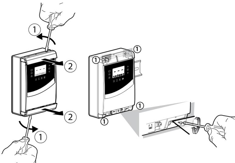
2.a: Remove the frames, loosen the screws (1) and open the panel
