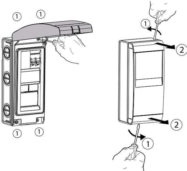
3: Raise the cover or remove the faceplates and unscrew the screws to remove the panel and open the module.
