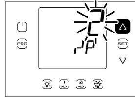
7. Press Set and UP/DOWN to set the desired value of the parameter.
