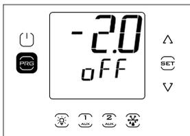
1. When first starting, the controller is OFF.
